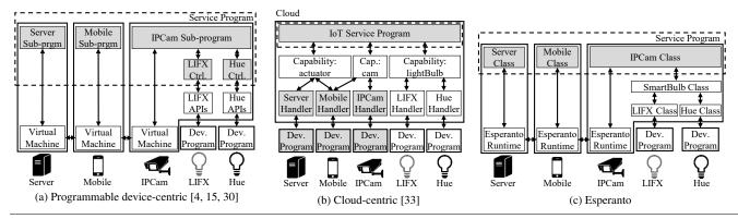
**Figure 2.** The overall structures of the baby monitor program (Figure 1) in different IoT frameworks. Here, the baby monitor program executes customized sub-programs for multiple programmable devices such as the IP camera, the server and the mobile, exploiting third-party devices such as Hue and LIFX smartbulbs. Gray boxes are programs that programmers need to write, and dashed boxes are integrated programming views that each framework provides.
