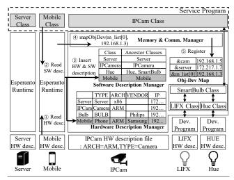
Figure 8. The overall structure of the Esperanto runtime
